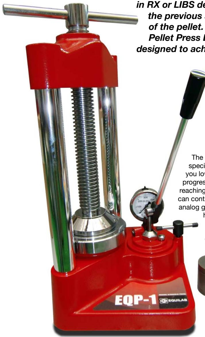
**Obtaining truly representative results in RX or LIBS depends very much on the previous step, the manufacturing of the pellet. The Hydraulic Manual Pellet Press EQO-1 has been specially designed to achieve high quality pellets, homogeneous and stable. Able to apply pressure up to 20 tons, it is simple and safe to manage, and it occupies very little room in the laboratory.**
