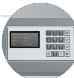
Example: The number of taps is 10, 500 and 1250, and the speed is 250 taps/min (3 mm drop height), according to **USP and Ph. Eur.**
